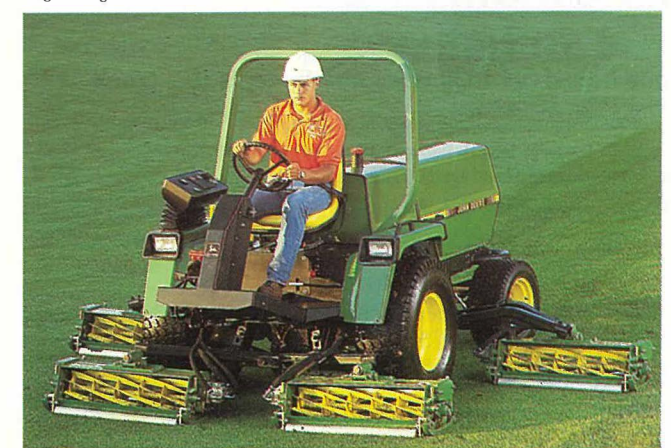
3325 Hydraulic Turf Mower. 28kW (38hp) diesel engine. Single lever lift for all five 30" cyls and standard hydraulic weight transfer system. 138" wide cut. Optional 6, 8 or 10 blade cutting units, solid or grooved front rollers and verti-cutter heads available.
