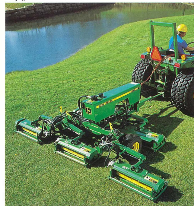
305 Gang Mower. Hydraulically driven (30-45hp). 5x30" cylinders, 142" wide cut. Optional 6, 8 or 10 blade cutting units; solid or grooved front rollers and verti-cutter heads available.
