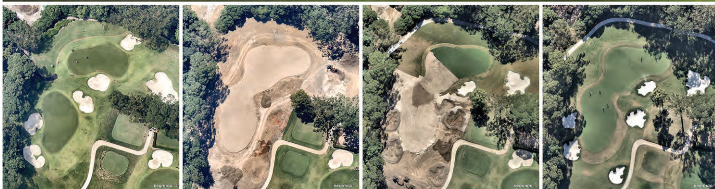
One of the biggest design changes and undertakings of the project was the construction of a new double green – 8 and 14 – which measures 1225m 2 . Pictured top is looking toward the green from the 8th tee, while the aerial photos show the complex before, during and after construction
